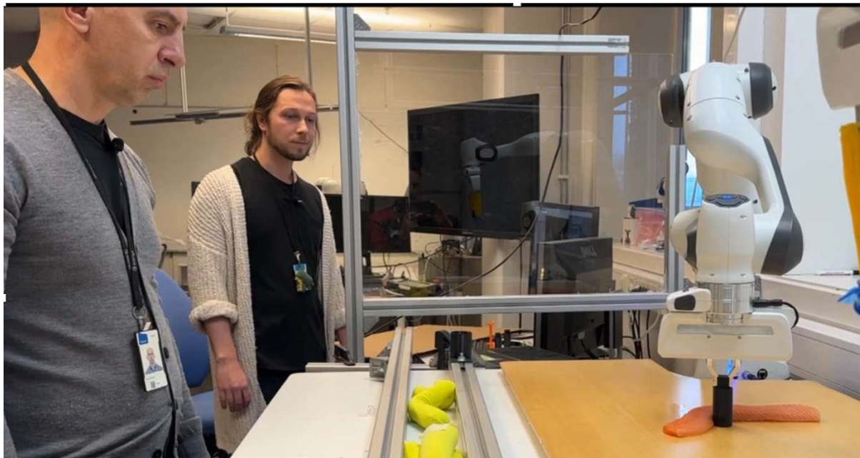
Figure 1 non-prehensile robotic manipulation of salmon loins - the agent is trained exclusively in simulation and is deployed zero-shot to the real world. Non-prehensile manipulation alleviates the need to grasp the objects unnecessarily and, in this way, achieve the task by being gentle to the product and avoiding the quality degradation during processing stages of salmon. From: Herland, S., & Misimi, E. (2025). Non-prehensile shape manipulation of elastoplastic objects with reinforcement learning. In Proceedings of the 2025 IEEE International Conference on Robotics and Automation (ICRA) (pp. 13204–13210). IEEE. https://doi.org/10.1109/ICRA55743.2025.11127639
