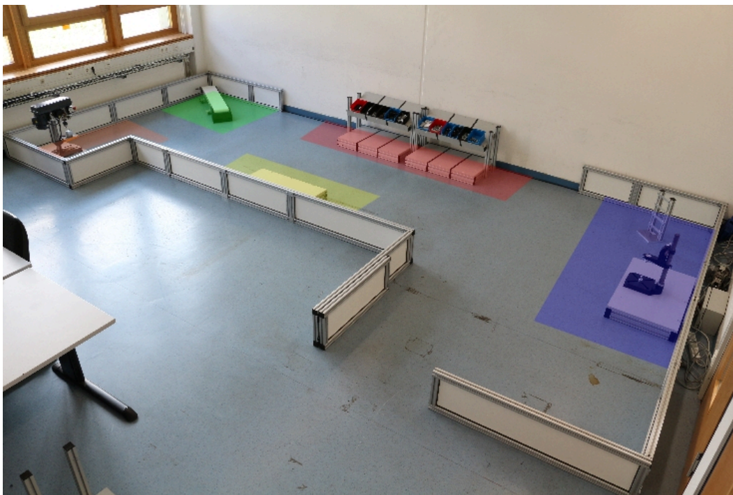
Figure 2: Example of the spatial areas in the ERL-PSR environment. The spatial areas are shelves (red), force fitting workstation (blue), conveyor belt (green), drilling workstation (orange) and assembly workstation (yellow).
