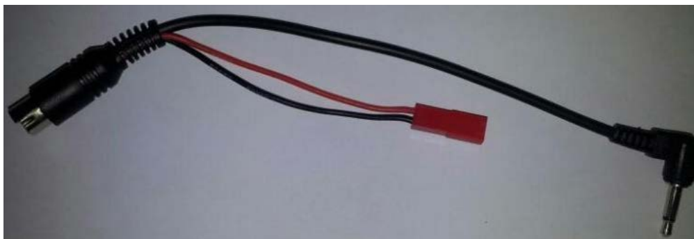
Figure 19. Buddy cable for EzUHF and Spektrum, JR, Turnigy, Graupner, Fly Sky and Hitec radios.
