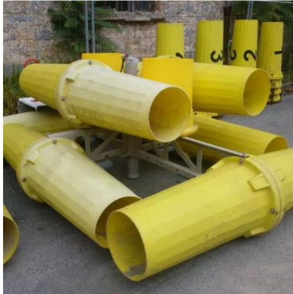
Figure 32. Piping assembly structure. The structure, composed of yellow pipes, has the following dimensions: 2 m (front area) x 3 m x 1.8 m (height).
