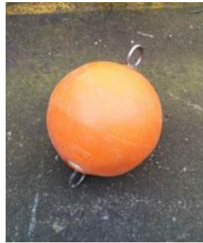
Figure 31. Image of the buoy without a number (gate). The OD of the sphere is 30 cm.
