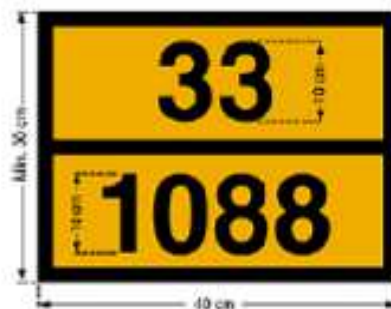
Figure 36. Example of an ERICard that will be positioned on the wall behind each valve.
